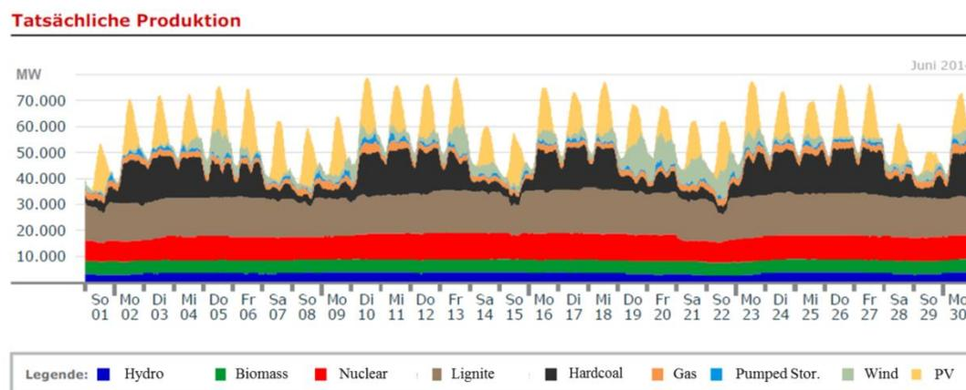
Fig.3. Electricity generation in Germany in June 2014 [2]
