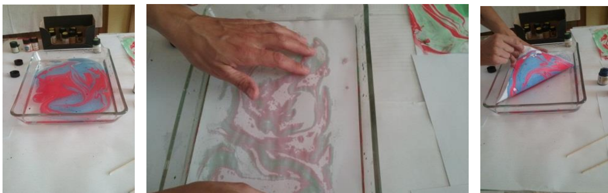
Fig.2. a) Mixed paints on the surface of water, b) Sheet flattened against the surface of water, c) The painted sheet lifted, fractal filaments become visible on the paper
