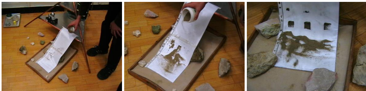
Fig.7. Experiment arrangement with various slope declinations of the magnetic carpet (a white sheet with invisible patterned magnet squares fixed inside). Left: the carpet is at a small angle, almost horizontal slope. Middle: dispersion and adhesion when the carpet is in position of a more elevated gentle slope position. Right: dispersion and adhesion onto a high-angle slope carpet [21]
