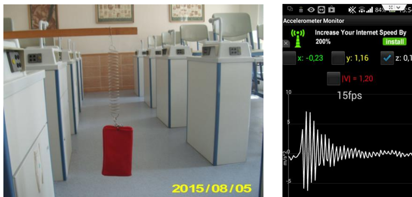
Fig.7. Acceleration-time graph of the damped oscillation
