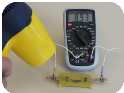
Fig.3. When warming up the Ge crystal, its electrical resistance decreases
