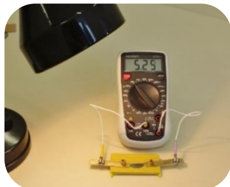
Fig.4. When illuminate the Ge crystal, its electrical resistance also decreases
