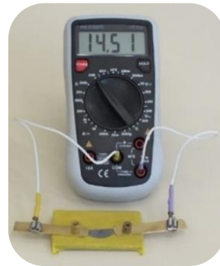
Fig.2. The multimeter shows us the resistance of the germanium at room temperature
