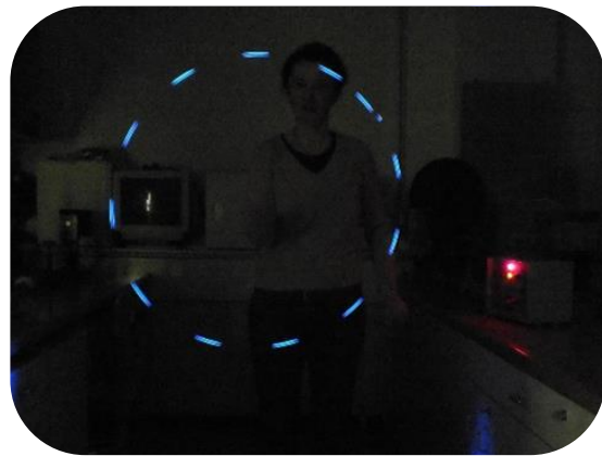
Fig.8. With alternating current we see an interruptedly lighting circle
