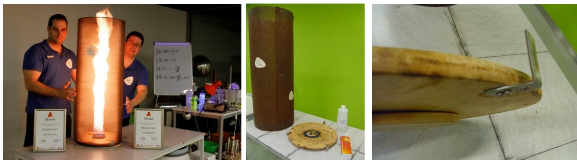
Fig.3. The self-developed fire tornado and the equipment
