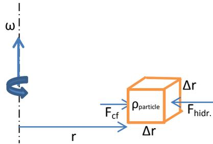
Fig.2. Air particle in the rotating flame column
