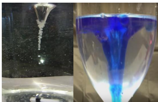
Fig.1. Water whirl Left panel: with plastic granules [photograph taken by the author in the von Karman Lab of ELTE]. Right panel: with coloured oil [10]
