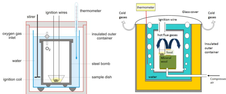
Fig.3. Left panel: Section view of a bomb calorimeter [18].
