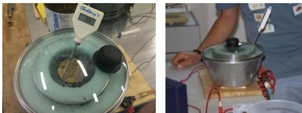
Fig.4. Left panel: Prototype of the modified bomb calorimeter showing the flow of air bubbles in the water. Right panel: the apparatus used by students for a measurement.
