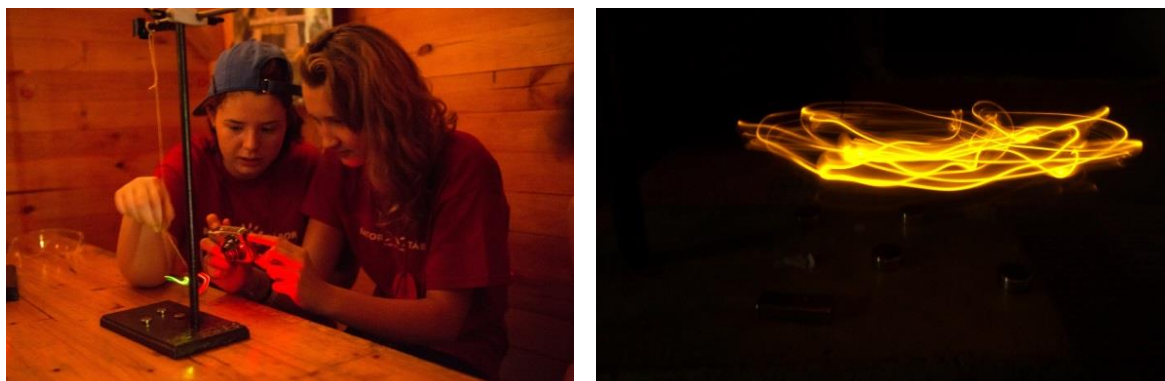
Fig.4. Experiment with magnetic chaotic pendulum. Left panel: The experimental set up. Right panel: Motion of chaotic pendulum visualized by yellow LED in 8 sec. exposure time
