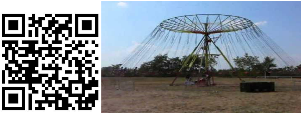
Fig.9. The QR Code seen in the picture helps us play the film and - with the help of a chronograph - measure the period time. The short film will also provide the measurements with further necessary information
