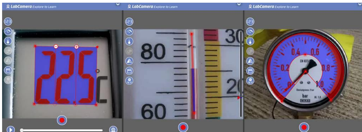
Fig.5. Instruments from which data can be logged into a computer with the help of Universal logger module
