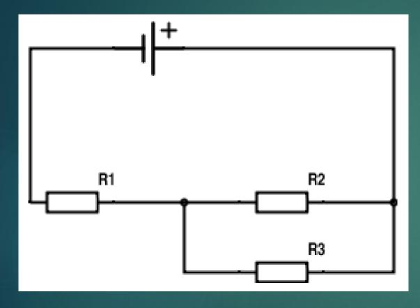
$$I_0 = \frac{U}{R_1 + \frac{R_3 \cdot R_2}{R_3 + R_2}}$$
